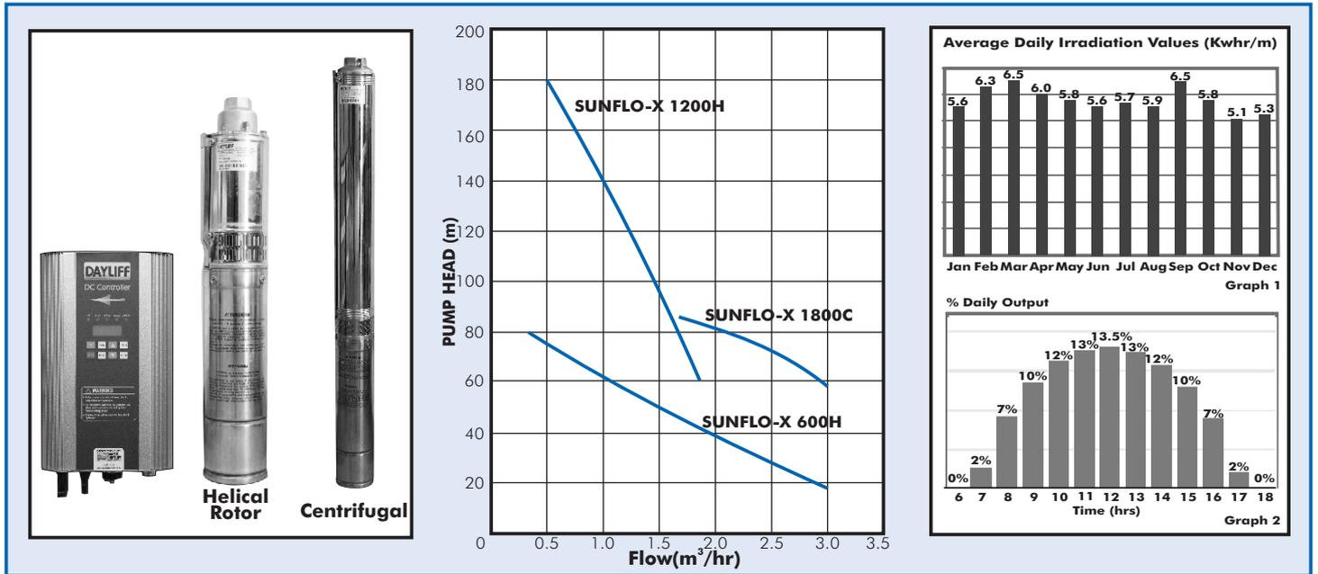
DAYLIFF SUNFLO-X Range of pumps are high specification solar powered centrifugal and helical rotor DC pumps specifically designed for borehole applications and feature a remote surface mounted controller. Pumps are constructed principally from AISI 304 stainless steel and are engineered to the highest standards to give serviceability, excellent efficiency, high reliability and long life. Helical rotor type are supplied with spare rotor.
