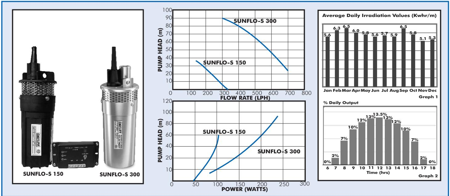
DAYLIFF SUNFLO-S series submersible pumps are designed for reliable small-scale water supply from boreholes and wells and are the ideal solution for remote pumping requirements in livestock watering, irrigation and general water supply applications. They are of positive displacement three-chamber diaphragm design and can run dry without damage. An internal bypass is also incorporated to prevent pump damage in the event of delivery cut-off.
