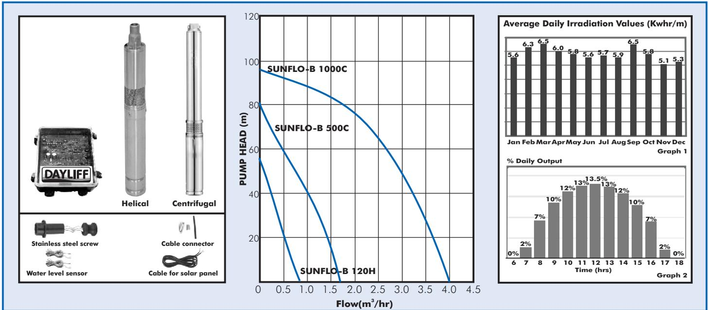
DAYLIFF SUNFLO-B pumps are specifically designed for PV solar powered water supply from wells and boreholes. They are of centrifugal and rotary screw design and material of construction for rotary screw design are principally stainless steel with a rubber stator while centrifugal design features noryl impellers and stainless steel chambers. Pumps are supplied complete with a controller, cable connectors, water level sensor, solar PV connecting cables and spare rotor for helical type.
