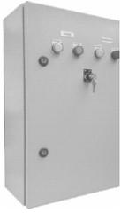
The Dayliff range of Auto Transfer Switches are specially designed for automatic switching of power supply between mains and generator inputs according to load requirements. They are specified for applications with Dayliff generators fitted with DSE modules and include motorised 4-pole breakers powered by a signal from the module. Manual power change over is also provided. The units are fitted with indicator lights to show active power and connection status.
