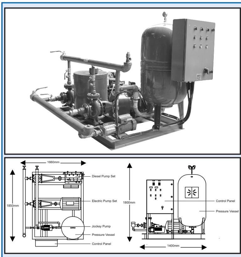
DAYLIFF FLA packaged Fire Sets are specially designed to provide automatic supply to multiple hose reel or sprinkler outlets for firefighting installations. Standard sets combine parallel duty diesel and electric powered supply pumps to ensure serviceability in all conditions as well as a jockey pump to maintain system pressure. Particular features include:-
