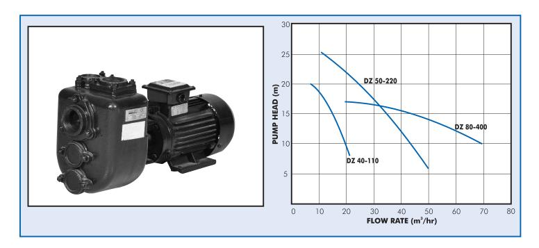
Dayliff DZ self-priming waste water pumps are of semi-open impeller axial flow type designed for pumping water containing high solid levels with particular application for site drainage, sewage and general effluent duties.
