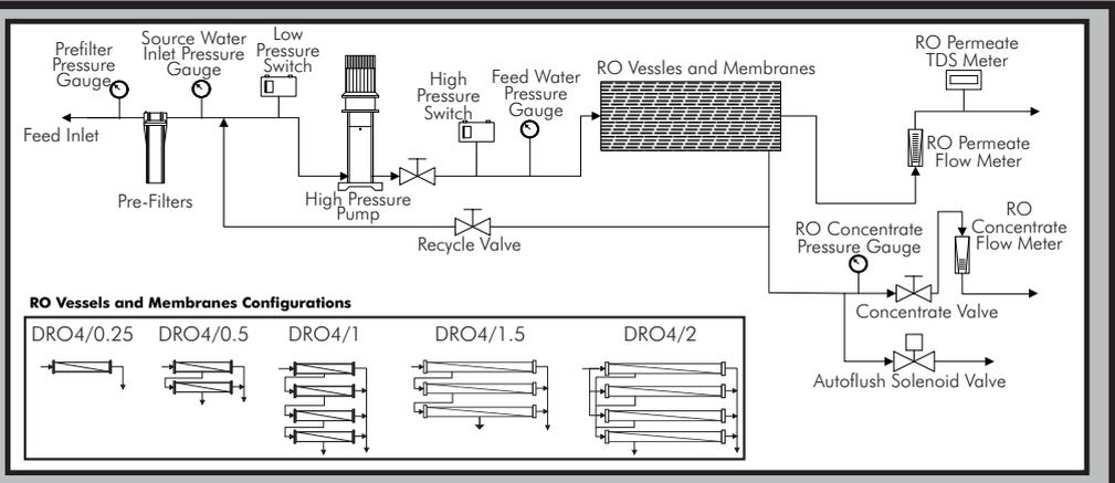
Reverse Osmosis is a proven technology to remove dissolved solids in water. At the heart of the system is the membrane, though the effectiveness of treatment relies on the correct matching of all components to provide an efficient treatment process, DAYLIFF plants being carefully engineered to provide reliability with the highest treated water quality.
