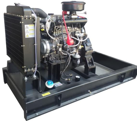
Dayliff DLY prime mover diesel engines are of 4-stroke, direct injection, water cooled design suitable for a wide range of stationary industrial and agricultural applications including water pumps, firesets and generators. All models are naturally aspirated cooled by forced water circulation and settable for fixed speeds between 1500 to 3000rpm.
