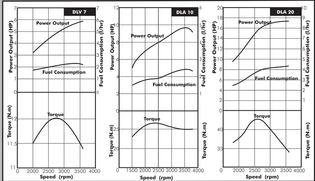
The Dayliff DL range of naturally aspirated engines are efficient and dependable designs suitable for a wide range of prime mover applications including pumps, generators, maize mills, chaff cutters, concrete mixers etc. Petrol and Diesel types are available as follows;
