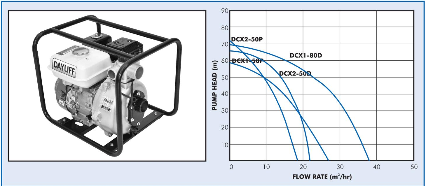
The DAYLIFF DCX range of portable high pressure engine are of self priming closed impeller centrifugal type suitable for high head water transfer, irrigation and fire fighting applications.
