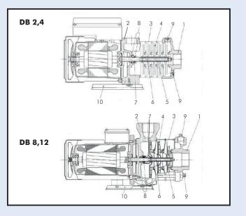
The DAYLIFF DB range of horizontal multistage centrifugal pumps are designed for continuous duty in various water transfer applications.
