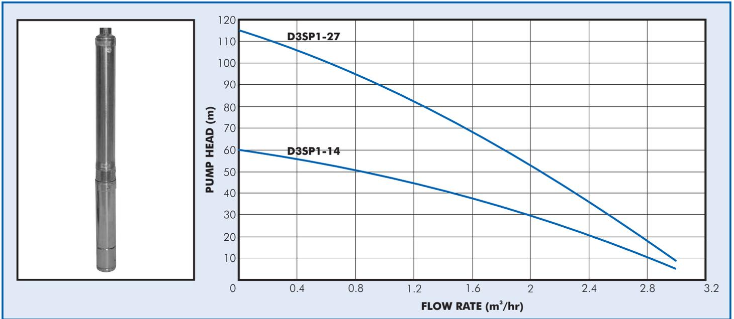
DAYLIFF D3SP1 pumps are compact 3" diameter submersible multistage centrifugal pumps specifically designed for small scale water supplies from boreholes and wells.
